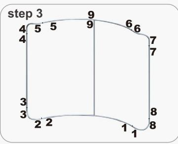
Connect all the pipes together, according to the sticker number on each pipe.
