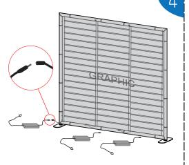
Connect the power line of the LED light panel
