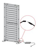
Connect the power line of the LED light panel
